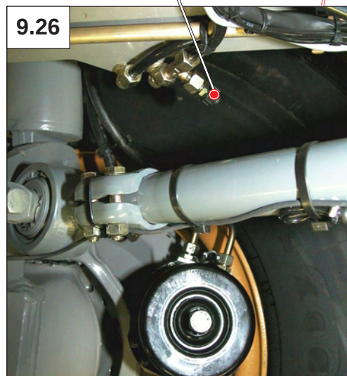
M2 measuring point parking brake pressure
