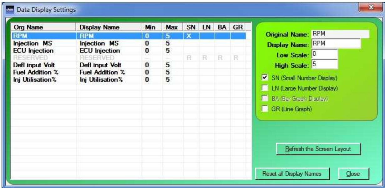
The Injection utilization display is very important. It tells you when the injectors 'max out': that is to say when the injectors are 100% ON, and you can't inject more fuel. If the engine requires more fuel, then it would run LEAN. This is OK at cruising, but dangerous at full throttle.
