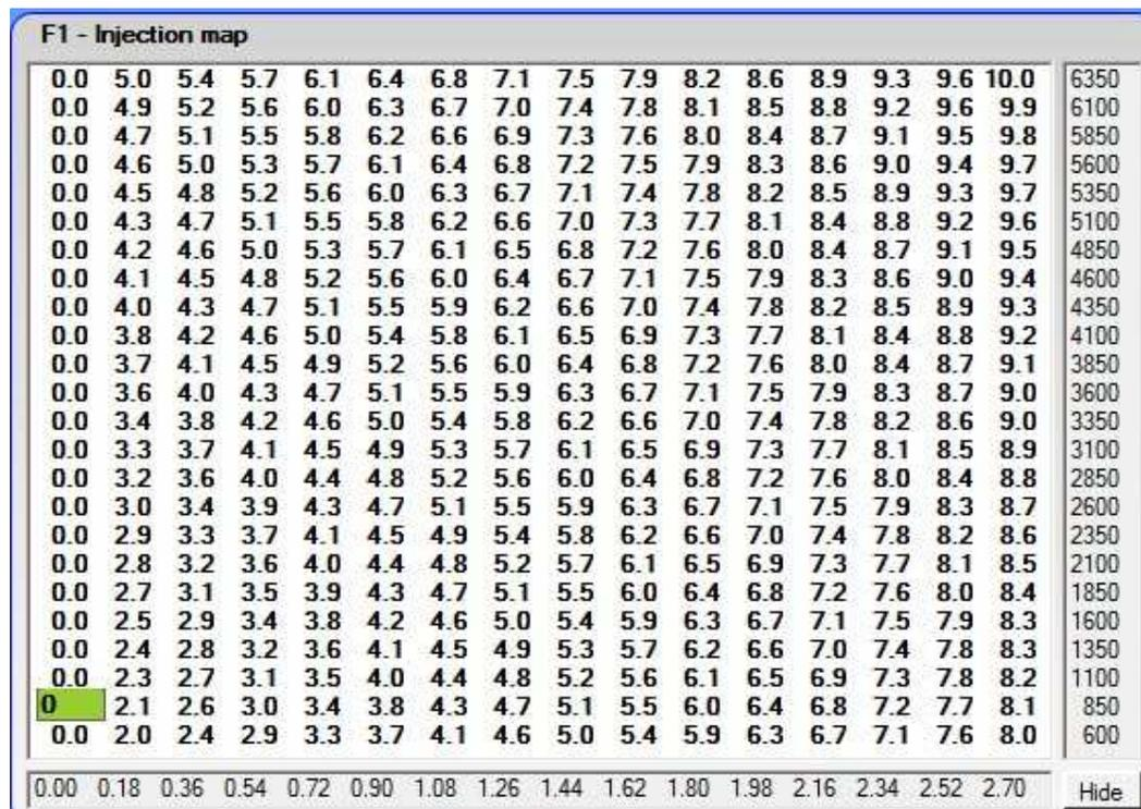
The screenshot shows a software window titled "F1 - Injection map". It contains a grid of numerical values representing fuel injection amounts. The grid has 16 columns and 20 rows. The first column is labeled "0.0" and the last column is labeled "6350". The rows are labeled with RPM values from 6350 down to 600. The values in the grid range from 0.0 to 10.0. A "Hide" button is visible in the bottom right corner of the window.
