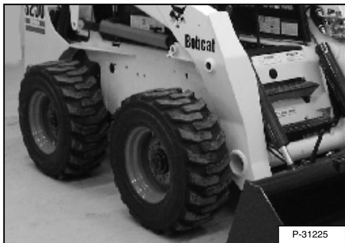
For the service interval to check the wheel nuts (See SERVICE SCHEDULE on Page PM-5). The correct torque is 142-156 Nm torque [Figure PM-52].
