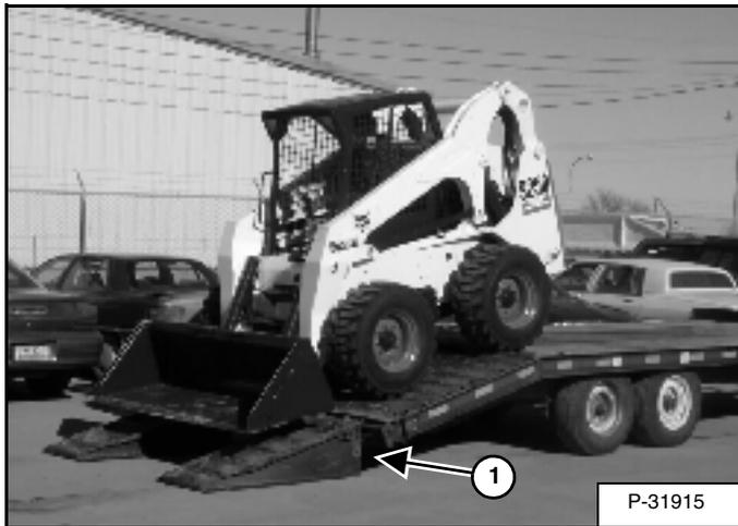
A loader with an empty bucket or no attachment must be loaded backward onto the transport vehicle [Figure OI-97].
