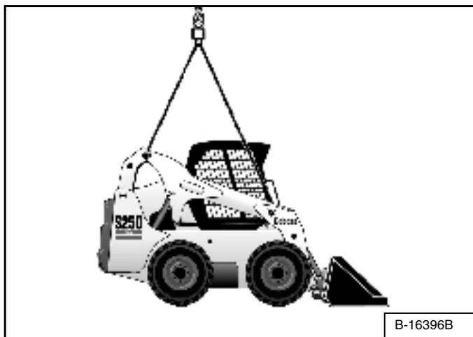
Attach cables or chains to lift eyes [Figure OI-100].
