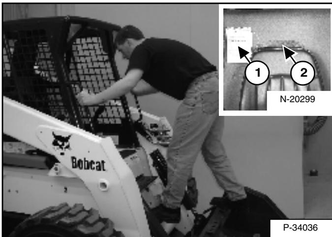
Use the bucket or attachment steps, grab handles and safety treads (on the loader lift arms and frame) to get on and off the loader [Figure OI-42]. Do not jump.
