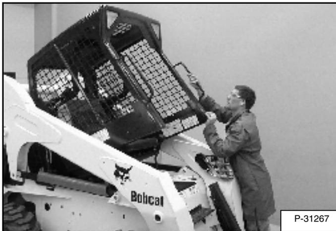
Lift on the grab handles and bottom of the operator cab [Figure PM-6] slowly until the cab is all the way up and the latching mechanism engages.
