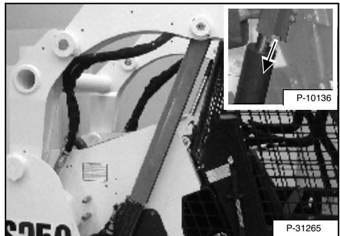
Lower the lift arms slowly until the lift arm support device is held between the lift arms and the lift cylinder [Figure PM-3]. The tabs of the lift arm support device must go under the cylinder (Inset) [Figure PM-3].
