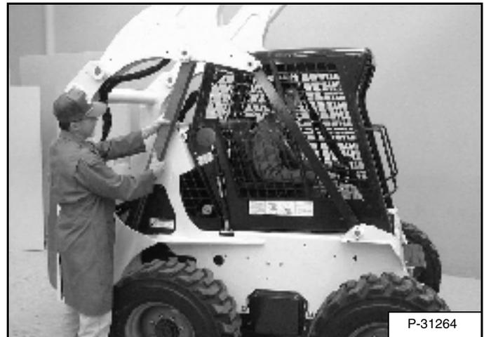
Have a second person install the lift arm support device over the rod of one of the lift cylinders [Figure PM-2].
