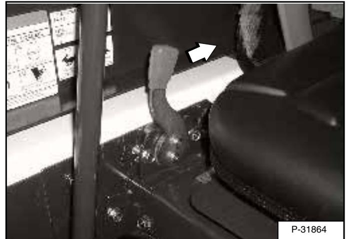
Pull the engine speed control fully backward [Figure OI-58] to decrease the engine speed.
