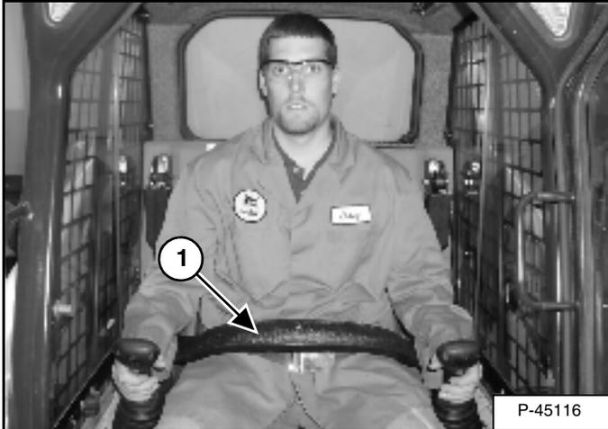
The seat bar restraint system has a pivoting seat bar with arm rests (Item 1) [Figure OI-22].
