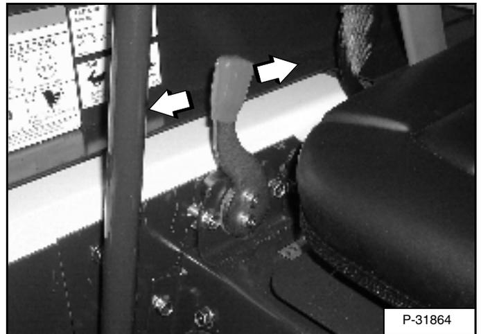
Set the engine speed control to the 1/2 speed position [Figure OI-48].
