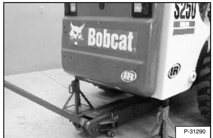
Install jackstands under the rear of the loader frame [Figure PM-4].
