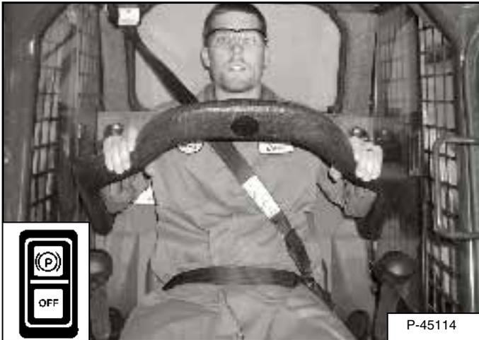
Lower the seat bar and engage the parking brake [Figure OI-47].
