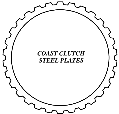
"STAMPED STEEL" COAST CLUTCH DRUM USED WITH 6.8L AND 7.3L "WITH" PTO OPTION
