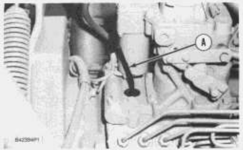
Timing Pin Installed (A) 6V6019 Timing Pin.
