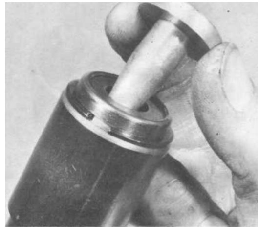
7.6c Do not omit restrictor, if removed
