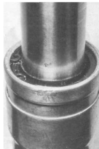
7.6e Renew seal and replace the circlip
