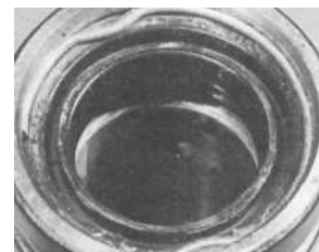
20.4b ... and displace circlip to permit removal of fork oil seal
