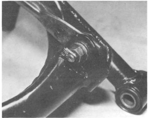
1 1.6 Check that torque arm mounting is secure
