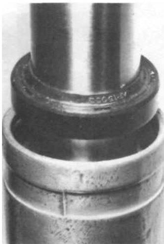
7.3 New seals should be fitted as a precaution
