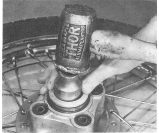
11.2c A large socket makes a useful drift
