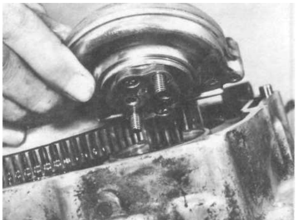
11.1b Pump can be lifted away as a unit
