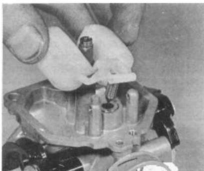
15.1 If float assembly is one-piece plastic item, incorrect float height can be cured only by renewing worn components
