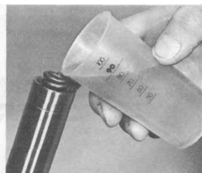
21.3b Refill fork leg with exactly the correct amount of oil
