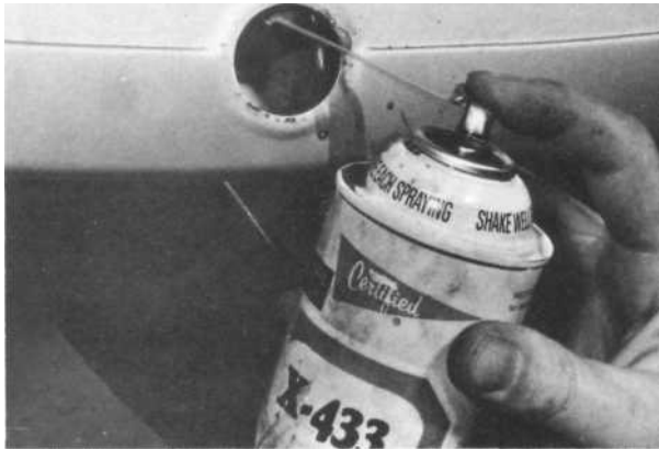
14.2a Plug can be removed for lubrication and chain tension check
