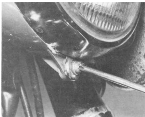
6.1 Lens/reflector unit is secured by screw through rim - early models
