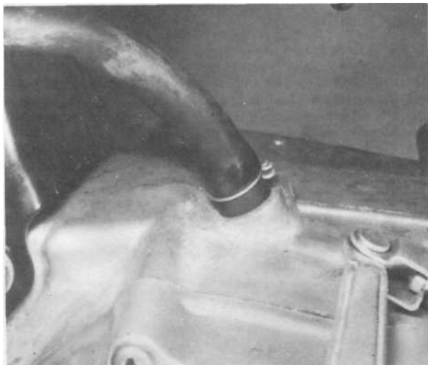
40.3a Push breather pipe over crankcase stub
