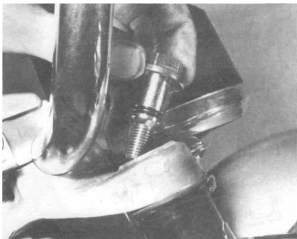
3.2 Remove fork top bolt to release yoke
