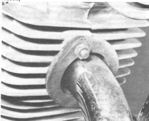
5.6a Remove exhaust pipe flange followed by .
