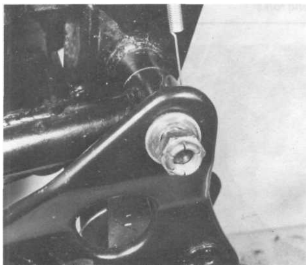
1 1.4a Slacken and remove pivot shaft nut
