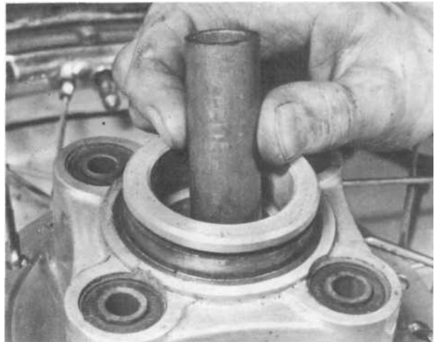
11.2a Spacer is fitted between wheel bearings
