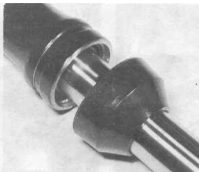
20.4a Remove dust seal from lower leg ...
