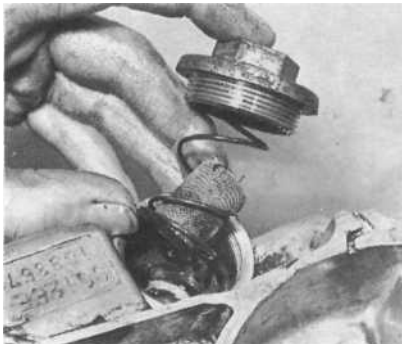
Strainer is easily removed for cleaning
