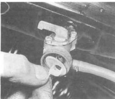
4.9a Ensure filter gauze is correctly located on refitting
