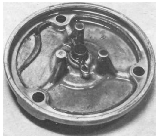
13.1 Centrifugal filter can be dismantled for cleaning
