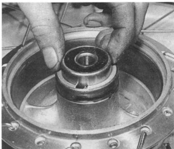
6.3b Bearing sealed surface must face outwards
