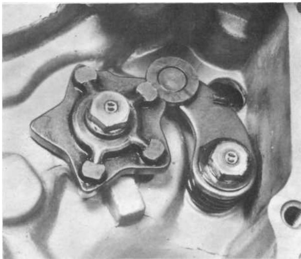
35.2c Fit camplate and tighten bolt
