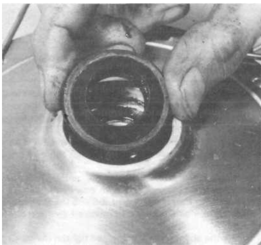
6.4 Renew seals together with bearings
