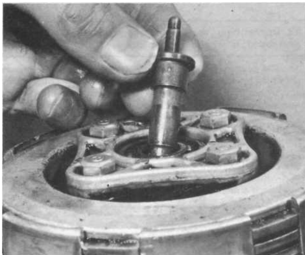
12.1a Remove the pushrod and pushrod seat
