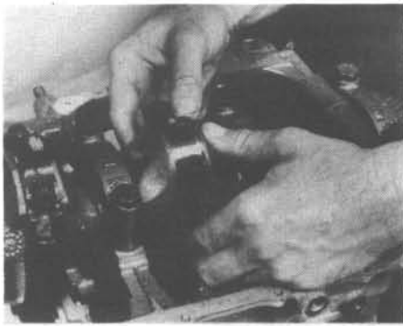
11.8 To prevent damage to the crankshaft journals and cylinder walls, slip sections of hose over the rod bolts before removing the pistons
