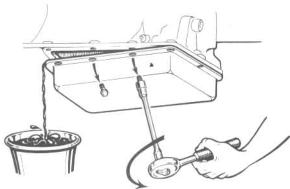
Fig. 1.18 Automatic transmission oil pan removal (Sec 27)
