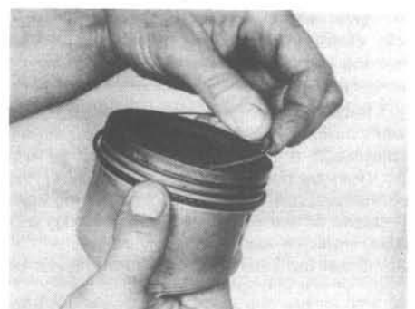
18.9B Do not use a piston ring tool when installing the oil ring side rails
