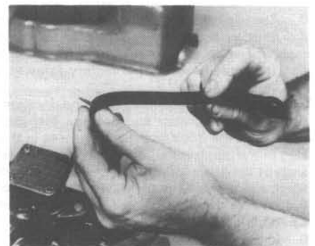
34.4 During installation the rubber tips on the front oil pan gasket should be pressed into the holes in the timing gear cover
