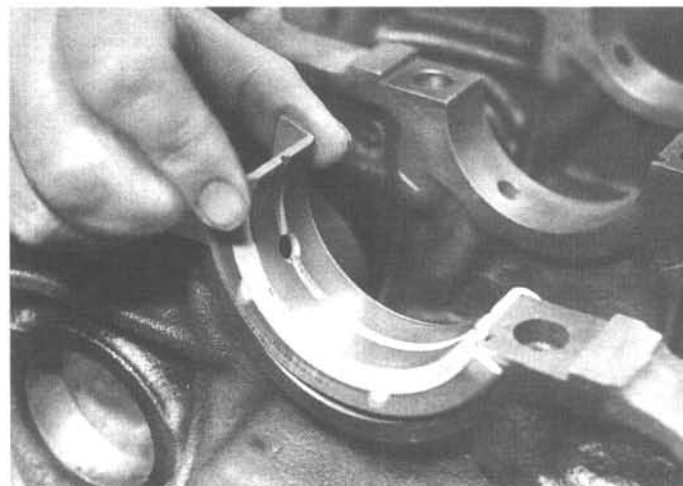
64.6 The thrust bearing must be installed in the number three cap and saddle the block on six-cylinder engines and number two on four-cylinder engines
