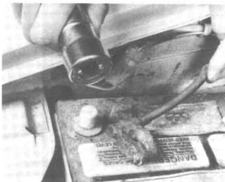
38.5C Cleaning the battery terminal post with a special tool
