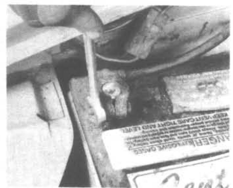
38.5B Removing the cable from the battery terminal post (always remove the ground cable first and hook it up last)
