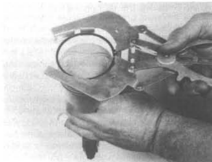
18.12 Installing the compression rings (note the special tool)
