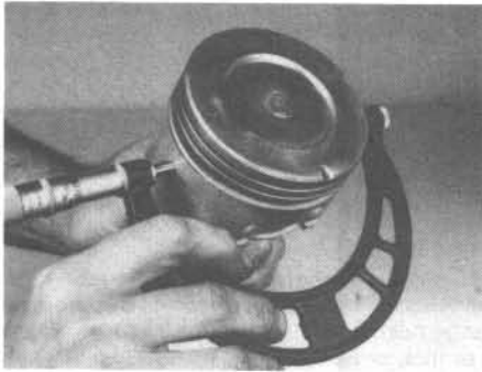
15.11 Measure the piston diameter directly in line with the piston pin hole (except on V6 engines)
