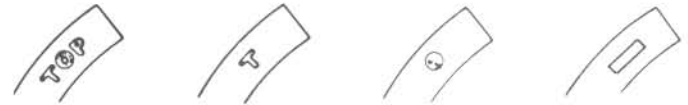
Fig. 2.8 Typical piston ring marks (always install the rings with the marks facing up) (Sec 18)
