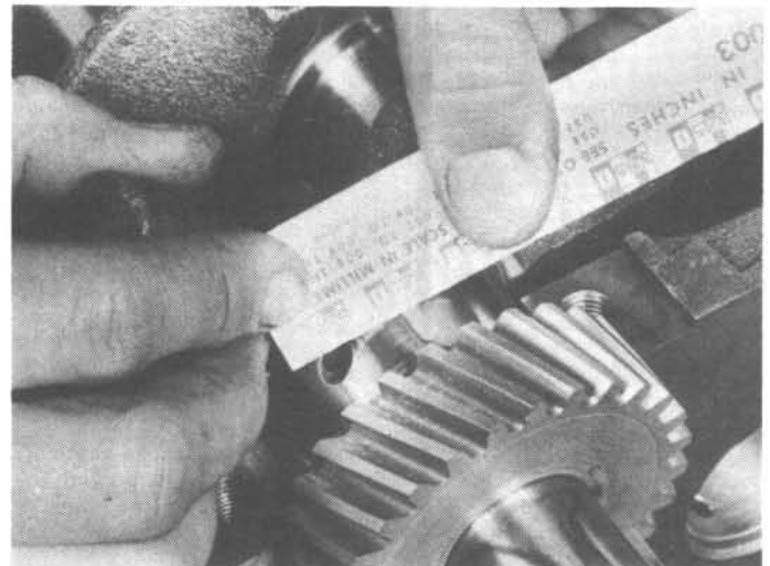
40.14 The oil clearance is obtained by comparing the crushed Plastigage to the scale printed on the container
