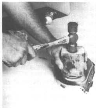
32.12 Using a block of wood to install the front oil seal in the timing gear cover
