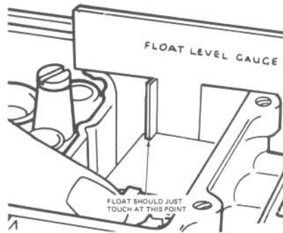
Fig. 4.31 Measuring the dry float level (2100/2150 carburetor) (Sec 13)
