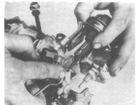
15.6 Lift off the idle speed solenoid/vacuum break assembly and disconnect the air valve rod from the outside vacuum break plunger
