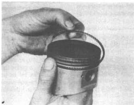
18.9A Installing the spacer/expander in the oil control ring groove
