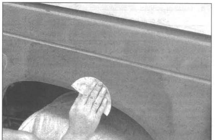
12 Finish sand the primer with very fine sandpaper (400 or 600-grit) to remove the primer overspray. Clean the area with water and allow it to dry. Use a tack rag to remove any dust, then apply the finish coat. Don't attempt to rub out or wax the repair area until the paint has dried completely (at least two weeks)
