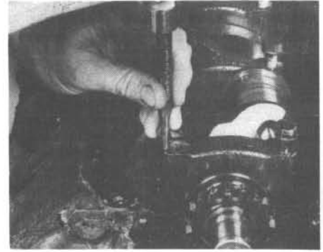
12.6 Mark the bearing caps with a center punch before removing them
