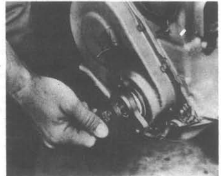
31.9 Pushing the hub onto the crankshaft with the hub bolt
