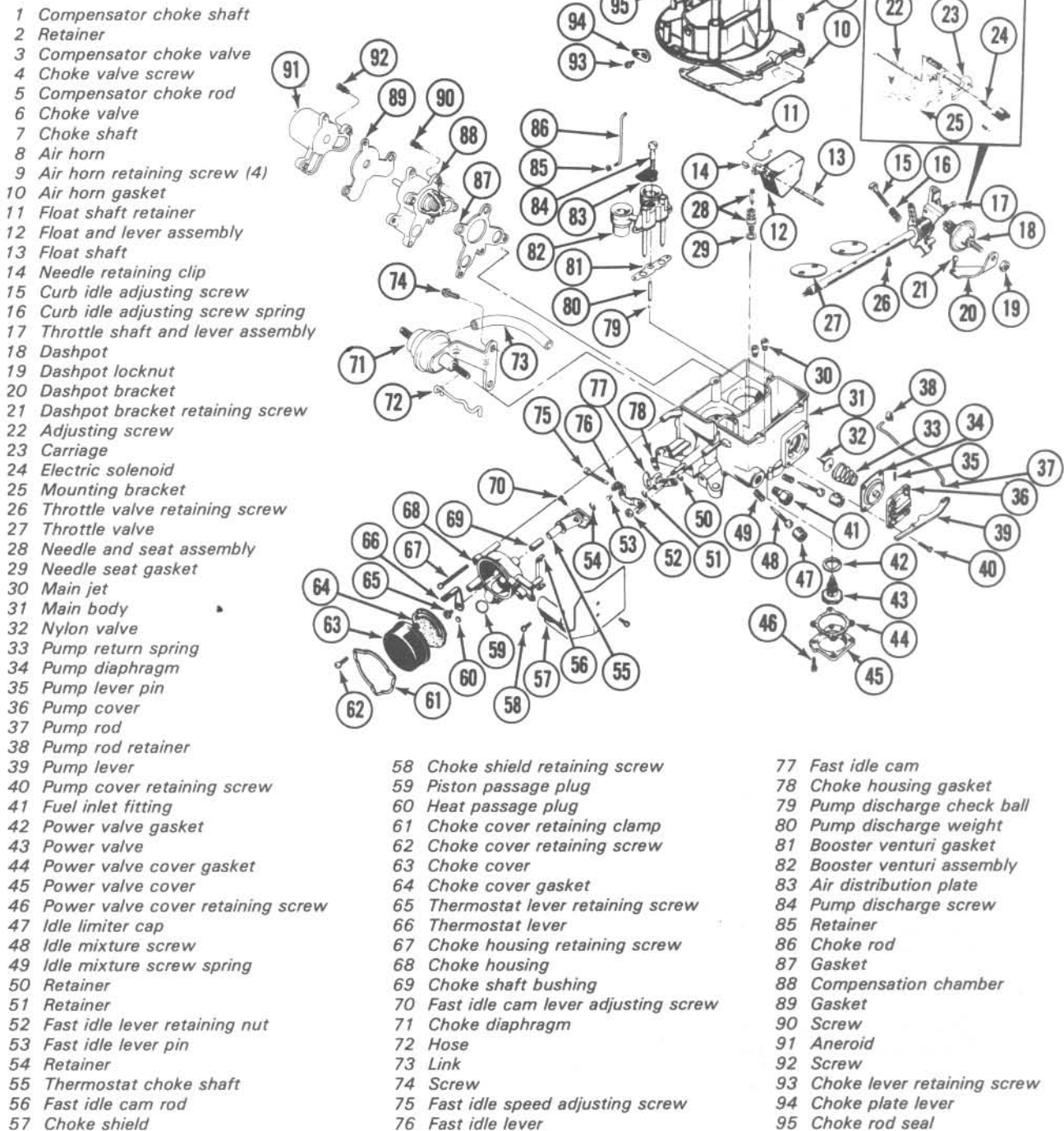
Fig. 4.26 Autolite/Motorcraft 2100/2150 carburetor components — exploded view (Sec 13)
