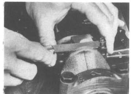
11.6 Checking connecting rod end play with a feeler gauge
