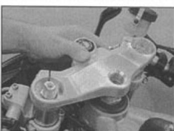
18.6b ... and draw the yoke up off the forks
