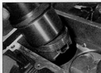
14.12 Carefully fit the liner down over the piston, making sure the rings enter correctly
