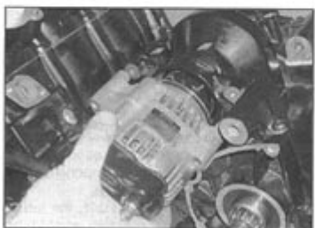
31.4b ... and remove the alternator
