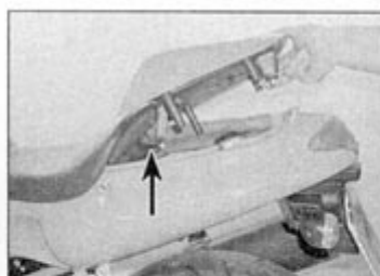
2.1b ... then draw it backwards and remove it, noting how the tab (arrowed) locates
