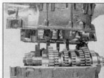
21.7 Carefully lift the lower half off the upper half, noting how the selector forks locate in the transmission shafts
