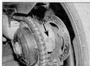
7.3b Slacken the clamp bolt (arrowed)
