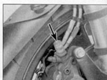
3.5a Brake hose banjo bolt (arrowed) – note the two hoses on the right-hand caliper
