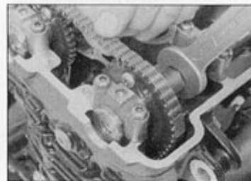
9.28 Slip the chain off the sprocket and turn the camshaft as required using a spanner on the cast hex
