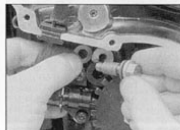
10.4 Locate the inner washer between the blade and the crankcase
