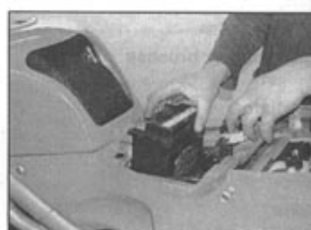
3.2c ... and remove the battery
