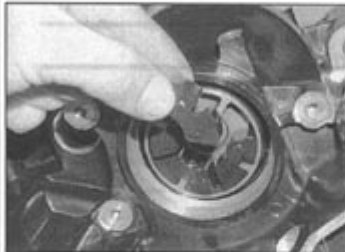
31.13 Fit the rubber dampers into the housing
