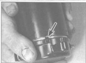
28.17b ... aligning the marks made on removal (arrowed)
