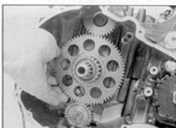
16.23b ... then slide the drive gear onto the shaft, making sure it engages correctly with both driven gears
