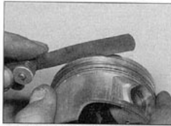
15.12 Measure the piston ring-to-groove clearance with a feeler gauge
