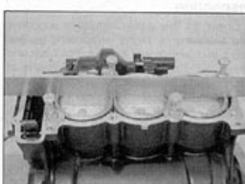
14.24 Check that the liners are all flush using a straight-edge
