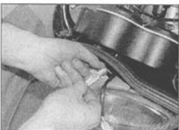
3.18c ... and disconnect the LED if fitted
