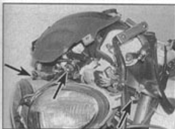
15.6 Instrument cluster nuts (arrowed) – Sprint ST
