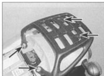
3.60 Luggage rack/tail light cover mounting bolts (arrowed)
