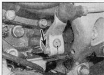
5.8 Make an alignment mark with the slit in the clamp, then unscrew the bolt (arrowed) and slide the arm (or lever) off the shaft
