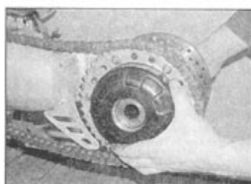
7.9a Slide the sprocket coupling onto the axle
