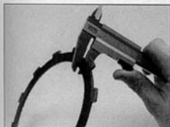
16.13 Measuring clutch friction plate thickness
