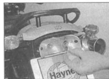
9.2c Push the bulb in and twist it anti-clockwise to release it
