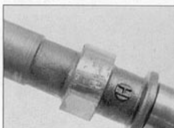
9.11b Check the lobes of the camshaft for wear – here's an example of damage requiring camshaft repair or renewal
