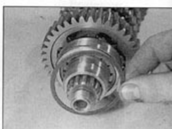
28.37c Fit the locating ring onto the end of the shaft, then fit the oil seal
