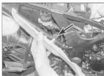
3.57b ... then undo the side panel screws and draw it away to release the peg from its grommet (arrowed)
