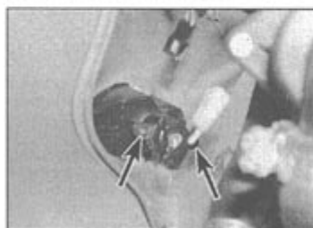
12.2 Undo the screws (arrowed) and remove the bulbholder
