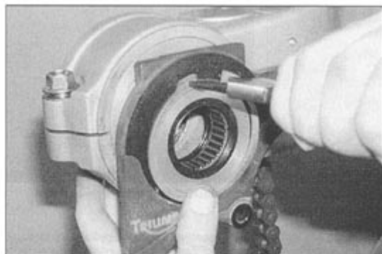
15.34a Remove the circlip ...
