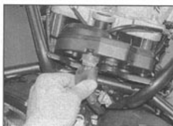
15.7a Pull back the rubber cover and disconnect the wiring connector
