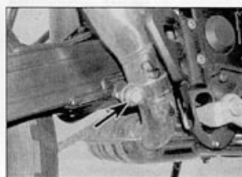
11.26 Slacken the clamp bolt (arrowed) ...
