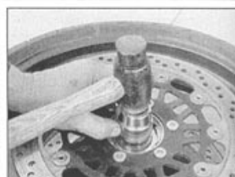
15.10 A socket can be used to drive in the bearing
