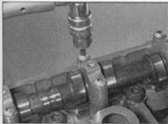
9.27 Tighten the cap bolts to the specified torque setting
