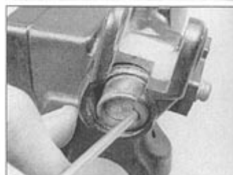
5.11c Remove the rubber boot from the end of the master cylinder piston ...
