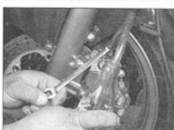
10.6c To bleed the brakes, you need a spanner, a short section of clear tubing, and a clear container half-filled with brake fluid
