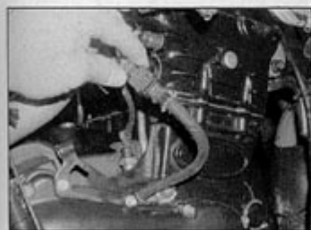
15.6a Disconnect the wiring connector ...
