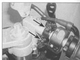
5.8 Front brake master cylinder clamp bolts (arrowed) - Daytona shown
