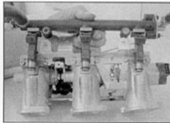
9.5b ... and carefully remove the fuel rail with the injectors attached (later model type rail shown)
