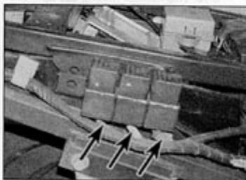
4.8b Relay pack – Sprint ST models. Identify the correct relay from the coloured identity tags (arrowed) – the cooling fan relay has a blue tag
