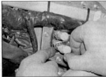
2.3 Press the retaining clip in to release the fuel hose
