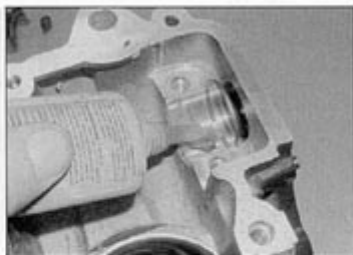
26.9 Apply the locking compound to the cutouts for the bearings
