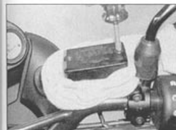
5.3b Slacken the reservoir cover screws
