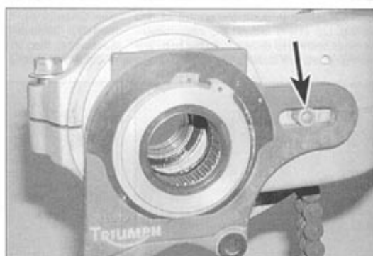
15.40 Locate the slot in the carrier over the peg (arrowed)
