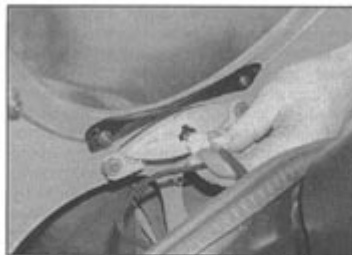
7.9 Release the bulbholder from the sidelight
