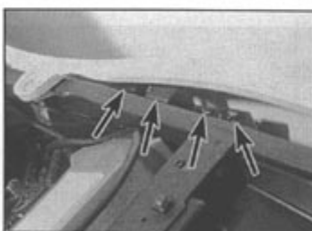
6.4c Relay pack (arrowed) – Sprint RS models. Identify the correct relay from the coloured identity tags
