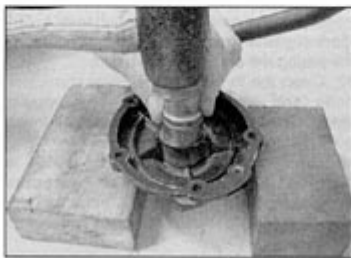
21.28c ... and press or drive it squarely into place ...
