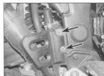
8.9c Master cylinder mounting bolts (arrowed) – Tiger
