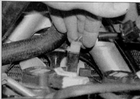
4.3 Cooling fan wiring connector – Daytona shown
