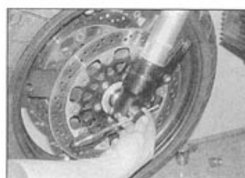
13.6b On Daytona and Speed Triple models, slide a screwdriver or bar through the hole in the end of the axle as a handle
