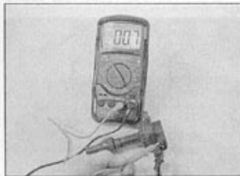
12.6 To test the coil resistance, connect the meter as shown
