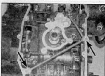
18.7b Unscrew the banjo bolts (arrowed) and remove the pipe ...
