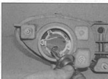
7.4c ... and remove the bulb
