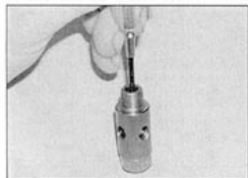
19.3a Push the plunger into the valve and check its action
