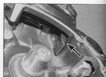
10.8b ... and make sure the blade hooks onto the crankcase correctly at the bottom
