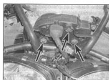
15.7b Undo the screws (arrowed) and remove the instruments
