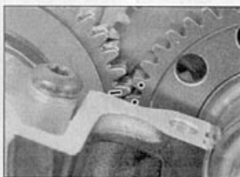
25.24 Crankshaft drive gear and balancer shaft driven gear alignment marks
