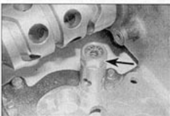
19.2 Unscrew the valve using a socket on the hex (arrowed)
