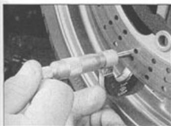
4.3 Using a micrometer to measure disc thickness
