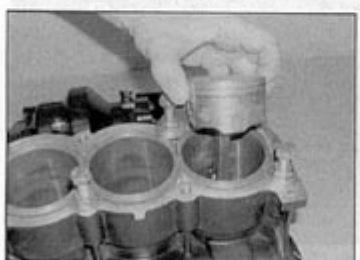
14.22a Carefully lower the connecting rod and piston into the liner ...
