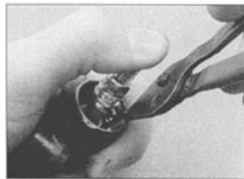
8.12a Depress the pushrod and remove the circlip
