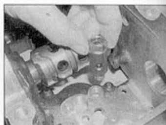
19.4 Install the valve and tighten it to the specified torque
