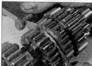
29.11a Measure the fork-to-groove clearance using a feeler gauge
