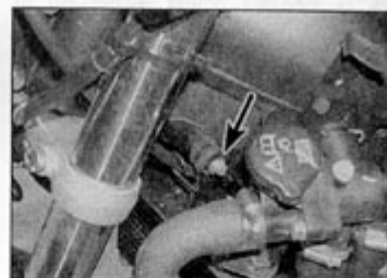
6.5b Radiator mounting bolt (arrowed) - there is one on each side - Sprint models
