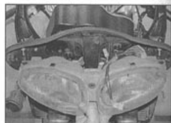
8.2c ... then displace the headlight ...
