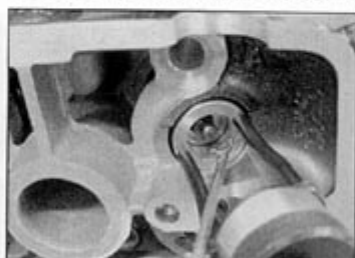
13.28b Compress the springs and install the collets, making sure they locate in the groove
