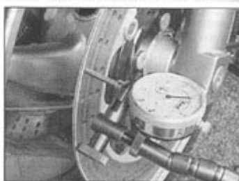
4.2 Set up a dial gauge with the probe contacting the brake disc, then rotate the wheel to check for runout
