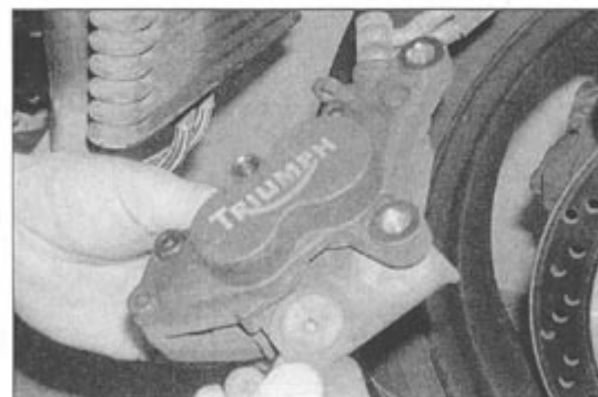
2.2d ... and remove the pads from the caliper
