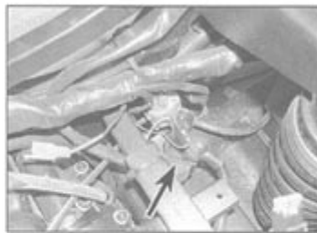
26.2b Starter relay (arrowed) - Tiger models
