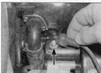
5.12 Pull back the rubber boot and unscrew the nut (arrowed) securing the lead
