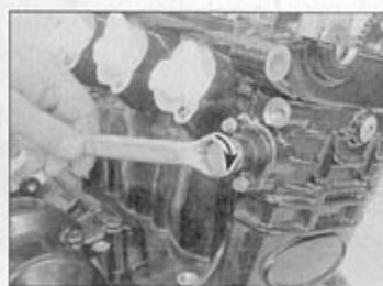
8.12 Turn the end bolt clockwise as described to release the plunger, and tighten it to the specified torque
