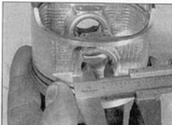
15.14c ... and the internal diameter of the bore in the piston
