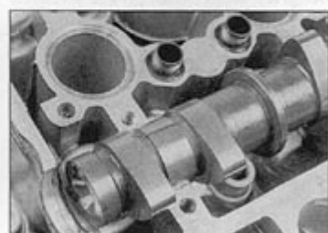
9.15 Lay a strip of Plastigauge across each bearing journal, parallel with the camshaft centreline
