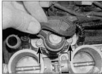
16.6 Idle air control valve screws (arrowed) – later type shown
