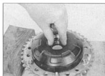
15.30 Press or drive the seal into the coupling
