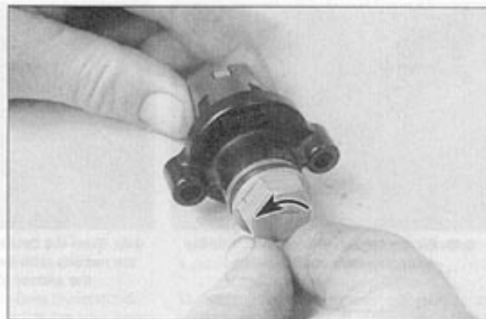
8.10b ... then turn the bolt anti-clockwise so that it threads into the plunger
