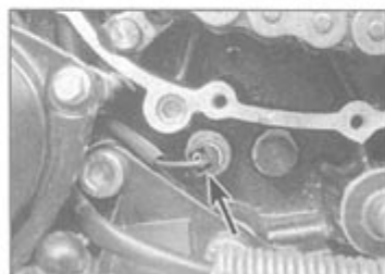
21.2 Disconnect the wiring connector (arrowed) from the switch
