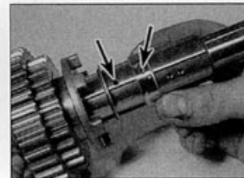
28.33b ... followed by the 4 th gear bush, aligning the oil holes (arrowed)
