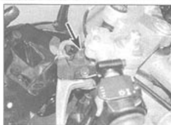
23.1 Clutch switch (arrowed)
