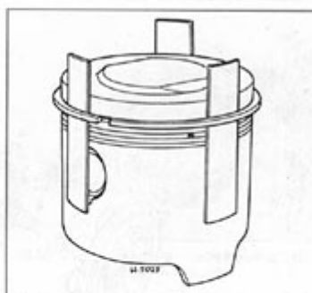
15.25b Old pieces of feeler gauge blade can be used to guide the ring over the piston
