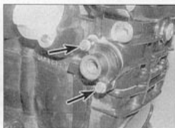
8.6 Unscrew the bolts (arrowed) and withdraw the tensioner body from the head
