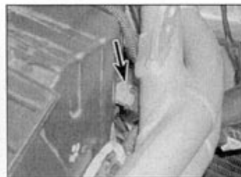
4.3a Intake air temperature sensor (arrowed)
