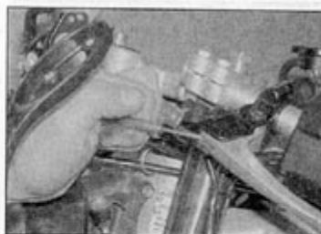
17.5a Draw the outer cable end from the adjuster and slip the inner cable out via the slots ...
