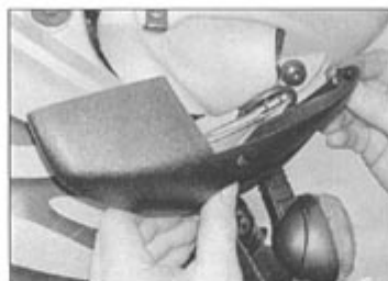
3.62b ... then displace the panel and disconnect the wiring connectors
