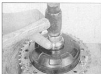
15.29 A socket can be used to drive in the bearing
