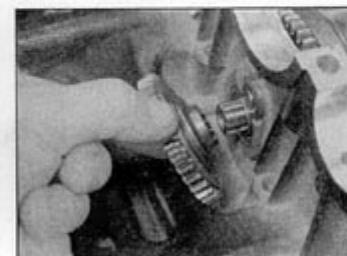
31.6f . . . and slide the gear off the shaft
