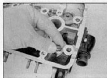
13.26b ... followed by the valve stem seal
