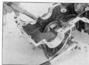
31.20 Counter-hold the bolt and tighten the nut to the specified torque
