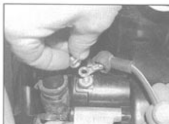
27.8 Secure the lead with the nut and fit the rubber boot
