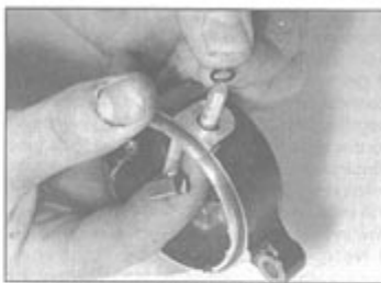
28.14b ... then fit the O-ring ...
