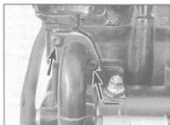
27.2b Undo the screws (arrowed) and remove the union
