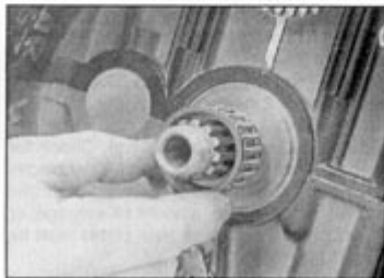
16.22a ... the needle bearing ...
