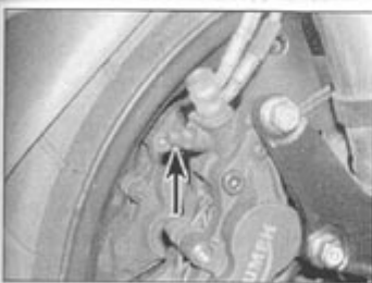
10.6a Front brake caliper bleed valve (arrowed) – Daytona, Speed Triple and Sprint models
