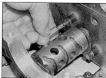
29.22b ... then rotate it to the position shown and install the screws
