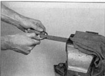
15.19 Ring end gap can be enlarged by clamping a file in a vice and filing the ring ends
