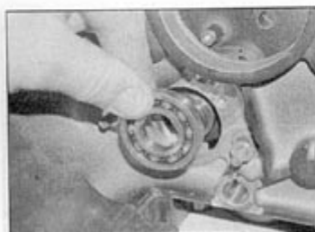
29.7b Remove the bearing, sliding the selector drum against it to dislodge it...
