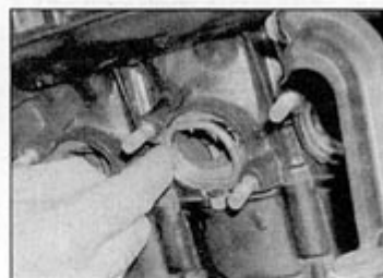
11.9 Smear the gaskets with grease to stop them falling out
