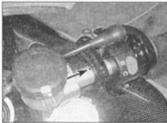
5.21 Align the mating surfaces of the clamp with the punchmark (arrowed) on the handlebar
