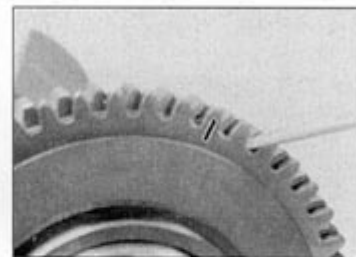
25.23b ... use a screwdriver between the teeth as a lever to align them
