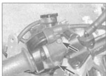
20.3a Right-hand switch housing screws (arrowed) – Daytona shown
