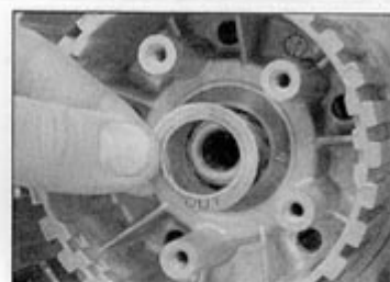
16.26b ... then fit the washer with the OUT mark facing out
