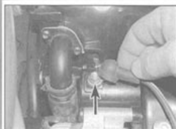
27.3 Lift the rubber cover, then unscrew the nut (arrowed) and detach the lead
