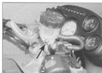
5.7 Reservoir mounting bolt (arrowed) - Sprint shown
