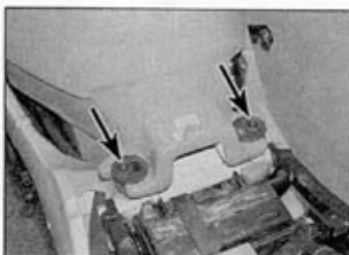
2.16b Rear mounting screws (arrowed)
