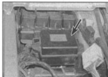
5.1a Fusebox (arrowed) – Daytona and Speed Triple models
