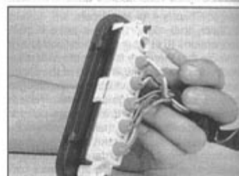
16.1h ... then pull out the bulbholder to access the bulb
