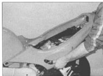
3.30c ... and remove the seat cowl
