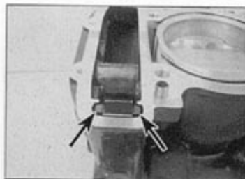
10.8a Locate the lugs in the cutouts (arrows) ...
