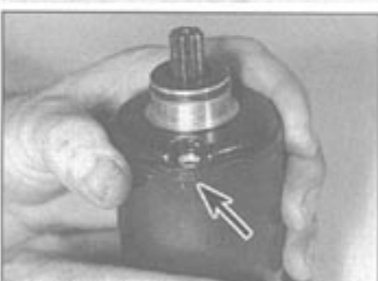
28.18 Fit the front cover, again aligning the marks made on removal (arrowed)
