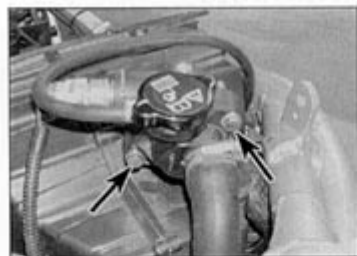
5.8 Thermostat cover bolts (arrowed) – Daytona shown
