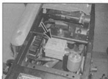
5.1c Fusebox (arrowed) – Tiger models
