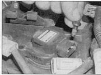
5.18b ... then undo the screws securing the coil to the valve cover ...
