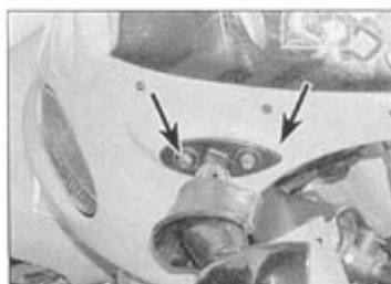
4.3c Mirror mounting bolts (arrowed)
