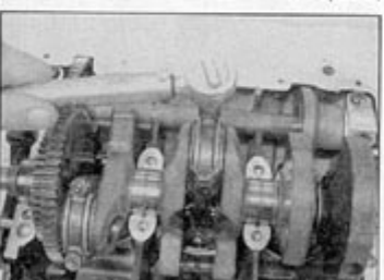
24.26d ... and tighten them first to the specified torque ...
