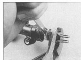
8.10 Hold the clevis and slacken the locknut
