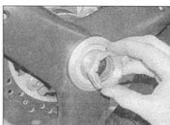
14.3b ... then unscrew the nut ...
