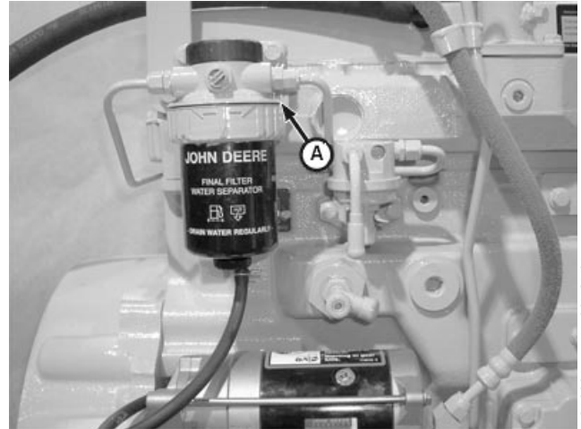
Final Fuel Filter Base
