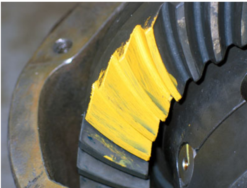
Figure 32 – Coast-side contact pattern - top / toe. Dark area illustrates contact pattern on coast-side is at the top and towards the toe of the teeth. Pinion depth must be significantly increased and backlash set to spec
