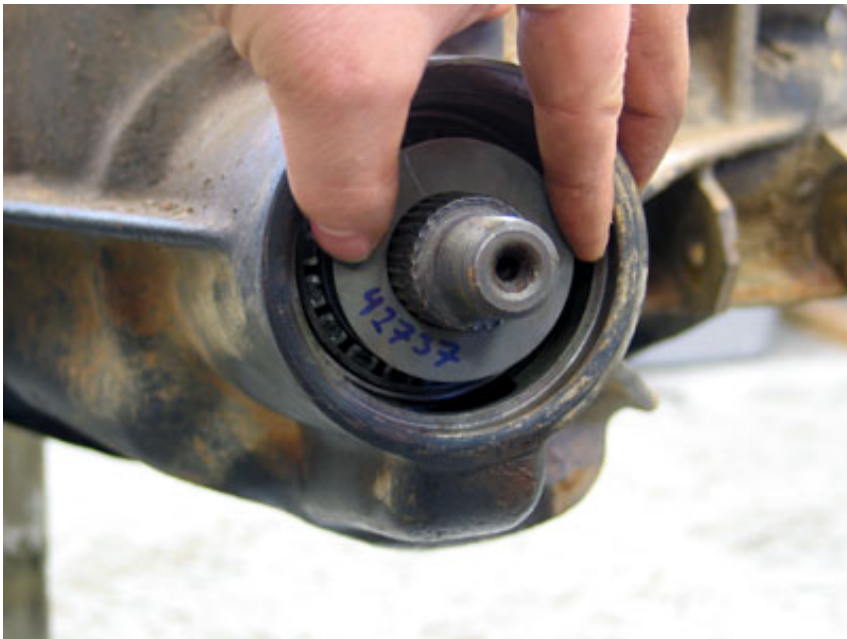
Figure 24 – Installing thrust washer on pinion
