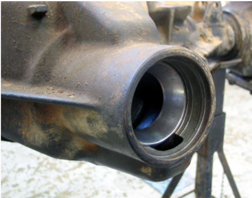
Figure 20 – Installed outer pinion-bearing cup
